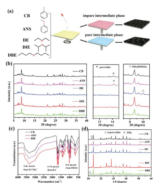
Fig. 1 (a) Schematic representation of the antisolvent-assisted perovskite deposition process, with chemical structures of the antisolvents used in this study. (b) XRD patterns and (c) FTIR spectra of the intermediate phases obtained from the  $Cs_{0.05}(MA_{0.17}FA_{0.83})Pb(I_{0.83}Br_{0.17})_3$  powder treated with the various antisolvents. (d) XRD patterns of the  $Cs_{0.05}(MA_{0.17}FA_{0.83})Pb(I_{0.83}Br_{0.17})_3$  films prepared using CB, ANS, DE, DIE, and DBE as antisolvents.
