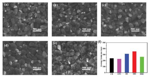
Fig. 2 (a-e) Top-view SEM images of the  $Cs_{0.05}(MA_{0.17}FA_{0.83})Pb(I_{0.83}Br_{0.17})_3$  films prepared using (a) CB, (b) ANS, (c) DE, (d) DE, and (e) DBE as antisolvents. (f) Average grain sizes of the  $Cs_{0.05}(MA_{0.17}FA_{0.83})Pb(I_{0.83}Br_{0.17})_3$  films prepared using the various antisolvents.
