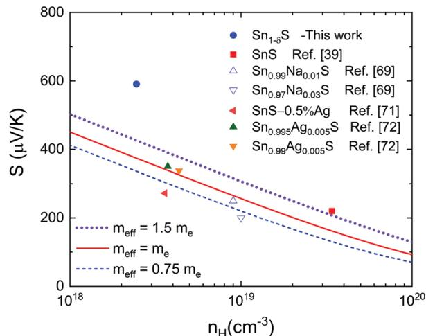
Fig. 9 Pisarenko lines for different effective masses at room temperature showing the single parabolic band model prediction for the Seebeck coefficient versus carrier concentration ( $n_H$ ) in comparison with our measurement and literature data.
