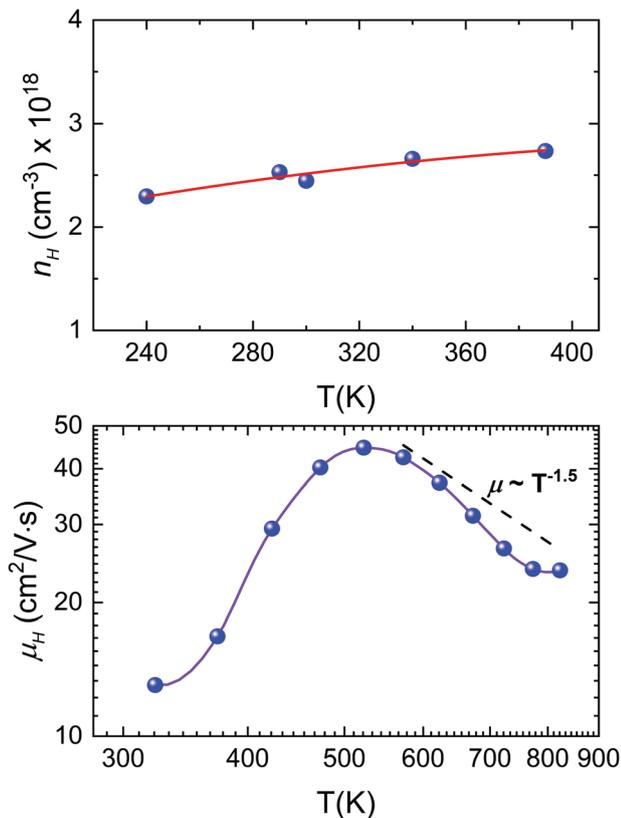
Fig. 8 (a) Temperature dependence of the Hall carrier concentration ( $n_H$ ). (b) Temperature dependence of the Hall carrier mobility ( $\mu_H$ ) of  $\text{Sn}_{1-x}\text{S}$ . The Hall carrier density of  $\sim 2.5 \times 10^{18} \text{ cm}^{-3}$  measured at room temperature is assumed to be unchanged up to 823 K. The solid lines are a guide to the eye. The dotted line corresponds to the  $\mu \sim T^{-1.5}$  temperature dependence.
