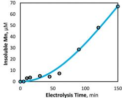
Fig. 7 Model and experimentally yielded results of insoluble manganese (Mn<sup>3+,4+</sup>) generation at 80 mA cm<sup>-2</sup> (left) and 40 mA cm<sup>-2</sup> (right) (pH = 7, [Mn<sup>2+</sup>]<sub>0</sub> = 175  $\mu$ M, T = 21.0  $\pm$  0.8 °C).
