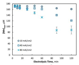
Fig. 2 Removal of aqueous manganese (Mn<sup>2+</sup>) with electrolysis time and current densities of 10, 40 and 80 mA cm<sup>-2</sup> (pH = 7, [Mn<sup>2+</sup>]<sub>0</sub> = 175  $\mu$ M, T = 21.0  $\pm$  0.8 °C).
