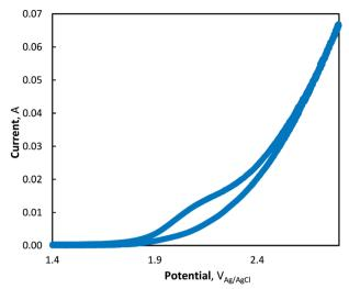
Fig. 3 Cyclic voltammogram of MnCl<sub>2</sub> at pH = 7 (phosphate buffer) and 10 mV  $\rm s^{-1}$  scan rate.
