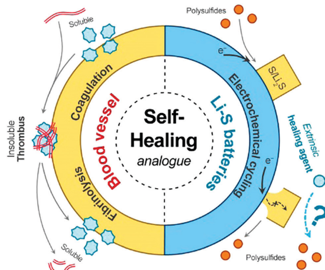
Fig. 25 Schematic of healing mechanism for sulfur particle cathodes. (left side) Simplified schematic of coagulation cascade toward formation of thrombus (blood clot) and fibrinolysis of thrombus into soluble fibrin fragments, which are modulated by two trypsins: thrombin and plasmin; (right side) schematic of deposition and dissolution of micrometer-sized sulfur/Li 2 S particles with limited electrical contact, hindering full electrochemical utilization. To enable the stable and reversible utilization, a complementary route is introduced, through chemical reactions between an extrinsic healing agent in solution and insoluble sulfur compounds. Reprinted with permission from ref. 413. Copyright 2017 American Chemical Society.
