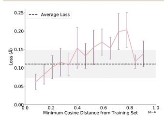
Fig. 4 Minimum cosine distance of test set from training set using learned embeddings from the GNN. Network loss increases as the distance between the test data point and training data increases. Each full bar corresponds to a single standard deviation, and the gray shading corresponds to a full standard deviation with respect to the average loss.
