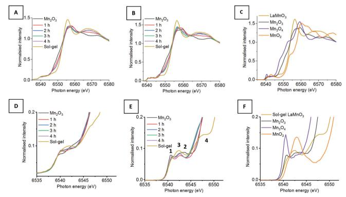
Fig. 1 (A) XAS Mn K-edge XANES compared to (B) HERFD-XANES of time-slices during the mechanochemial synthesis if LaMnO<sub>3</sub> compared to (C) reference Mn(II), (III), (IV) oxides and sol-gel synthesised  $LaMnO_3$  with (D-F) their respective highlighted pre-edge region.
