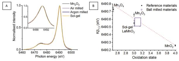
Fig. 8 (A) Mn Kβ XES mainlines of time-slices through the mechanochemical synthesis of LaMnO<sub>3</sub> from precursors La<sub>2</sub>O<sub>3</sub> and Mn<sub>2</sub>O<sub>3</sub> along with (B) which presents the  $K\beta_{1.3}$  max as a function of oxidation state, with a line of best fit calculated from the reference materials and used to calculate the oxidation state of the ball milled materials. 11
