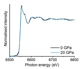
Fig. 4 In situ high pressure EDE spectra at 0 GPa and 20 GPa on  $La_2O_3$  and  $Mn_2O_3$  mixture after high energy ball milling for 30 min.
