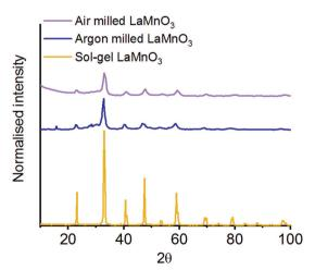
Fig. 5  $\,$  XRD patterns LaMnO $_3$  mechanochemically synthesised 4 h under atmospheric and inert (argon) conditions compared to the sol-gel synthesised perovskite.
