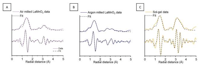
Fig. 6 Mn K-edge EXAFS data after 4 h of milling in (A) atmospheric and inert (B) milling conditions showing the magnitude and imaginary components of the  $k^2$ -weighted FT data and fits compared to (C) sol-gel synthesised LaMnO<sub>z</sub>.
