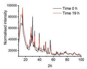
Fig. 3 XRD patterns at time 0 h and time 19 h after milling  $La_2O_3$  and  $Mn_2O_3$  with a PMMA vibrational mill.
