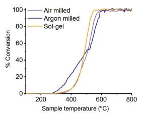
Fig. 10 Light-off curve of the percentage of deN<sub>2</sub>O to N<sub>2</sub> over LaMnO<sub>3</sub> catalysts synthesised by mechanochemistry and sol-gel synthesised with 0.5% N<sub>2</sub>O/He at 30 mL min<sup>-1</sup> with a pre-treatment of He at 30 mL min<sup>-1</sup>.
