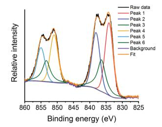
Fig. 12 La 3d XPS region for the argon milled catalyst showing the deconvoluted peaks at RT under a N2O atmosphere.
