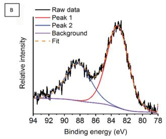
Fig. 11 (A) Mn 2p region and (B) Mn 3s region for the argon milled catalyst at RT under a  $N_2O$  atmosphere.
