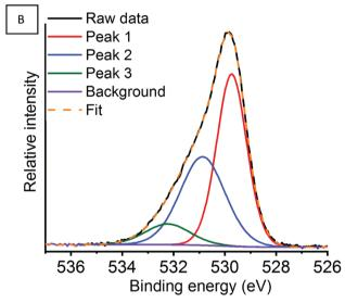
Fig. 13 O 1s region for the argon milled catalyst showing the deconvoluted peaks at (A) RT and (B) 600 °C under a N2O atmosphere
