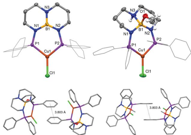
**Fig. 1** Top: Molecular structures of **1** (left) and **1-MeOH** (right) with thermal ellipsoids at the 50% probability level. Phenyl groups are depicted as wire frames, and hydrogen atoms except for NH and OCH<sub>3</sub> were omitted from the figures. Bottom: Intermolecular  $\pi$ - $\pi$  stacking in the extended XRD structure of **1-MeOH**.
