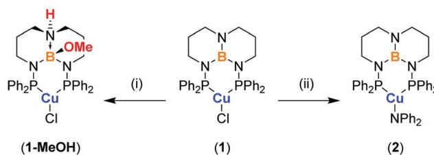
**Scheme 1** Structure of (<sup>Ph</sup>TBDPhos)CuCl (**1**) and synthesis of **1-MeOH** and **2**. (i) Excess MeOH at RT. (ii) Addition of 1 eq. of HNPPh<sub>2</sub> and KN(SiMe<sub>3</sub>)<sub>2</sub> in toluene at -78 °C.
