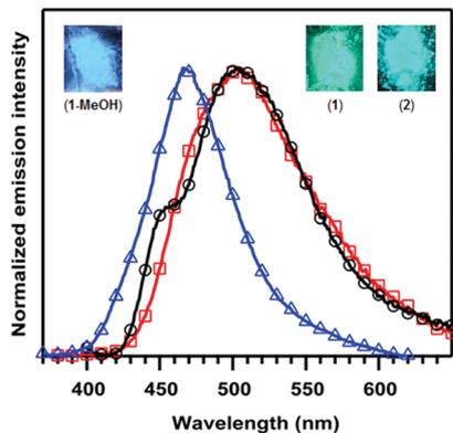
Fig. 2 Emission spectra for **1** (red;  $\square$ ), **2** (black;  $\circ$ ) and **1-MeOH** (blue;  $\triangle$ ) in the solid-state. Photoluminescence colours for **1**, **2**, and **1-MeOH** are provided at the upper right or left corners of the figure. Data were collected every 1 nm, and the symbols are present to help distinguish the overlaid plots.
