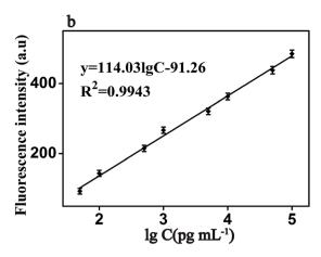
Fig. 6 (a) Fluorescence emission spectra of the biosensor in the presence of CRP with different concentrations: from bottom to top: 0 to 200 ng  $mL^{-1}$  (b) The fluorescence intensity as a function of CRP concentration. It shows the strong correlation between fluorescence intensity and CRP concentration, under both experimental conditions: RNA, 50 nM; P1, 20 nM; RNase H, 8 U; GO, 20  $\mu$ g mL<sup>-1</sup> and the emission wavelength of 519 nm. Error bars: SD, n=3.
