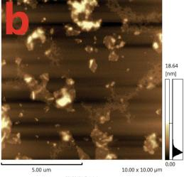
Fig. 3 The atomic force microscopy (AFM) images of different mixtures. (a) The AFM image of GO dripping directly on the surface of mica; (b) the AFM image of the mixtures of GO with microRNAs on the surface of mica. The concentrations of GO and microRNAs were 20  $\mu$ g mL<sup>-1</sup> and 20 nM, respectively. The volume of GO and microRNAs were both of 6  $\mu$ L.
