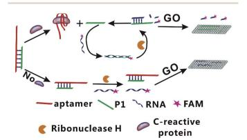
Fig. 1 Schematic illustration of the GO-based fluorescent aptasensor assay for the detection of CRP based on RNase H target recycling signal amplification (GO: graphene oxide; P1: DNA chain; FAM: 5carboxy-fluorescein).
