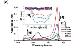
Fig. 4 UV-Vis spectra and CD spectra of MTC self-aggregates in 5  $\mu$ M dependent on the titration of NaCl (a and b) and LiCl (c), and all samples were tested after they stood for 2 hours at room temperature.
