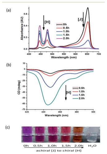
Fig. 2 The transformation from achiral J-aggregates to chiral Haggregates at room temperature. (a) UV-Vis spectra and (b) CD spectra in 5  $\mu$ M, all samples were tested after they stood for 2 hours; (c) the solution color changes in 100 µM in 2 hours
