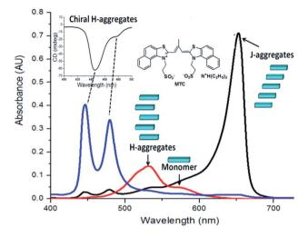
Fig. 1 The absorption spectra of 5 μM MTC in different states.
