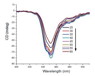
Fig. 3 The stability of MTC chiral H-aggregates in 5  $\mu$ M at various temperatures monitored by CD spectra, and all samples were tested after they stood for 0.5 hours at designated temperatures.
