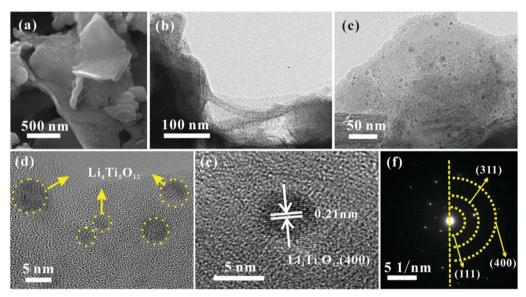
Fig. 4 Morphological structure of LTO QDs/CFs: (a) SEM image, (b and c) TEM images, (d and e) HRTEM images and (f) SAED image.
