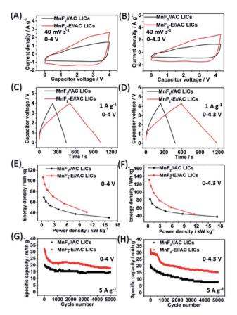
Fig. 5 CV plots at 40 mV s<sup>-1</sup> (A and B), GCD curves at 1 A  $g^{-1}$  (C and D), Ragone plots (E and F) and cycling behavior for 5000 cycles at 5 A g (G and H) of the MnF2 8#//AC and MnF2 8#-E//AC LICs under the voltages of 0-4 V and 0-4.3 V, respectively.
