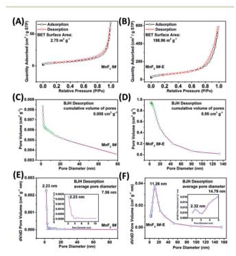
Fig. 3 N<sub>2</sub> isothermal sorption (A and B), pore volume (C and D) and pore size distribution (E and F) of the MnF<sub>2</sub> 8# and MnF<sub>2</sub> 8#-E samples, respectively.
