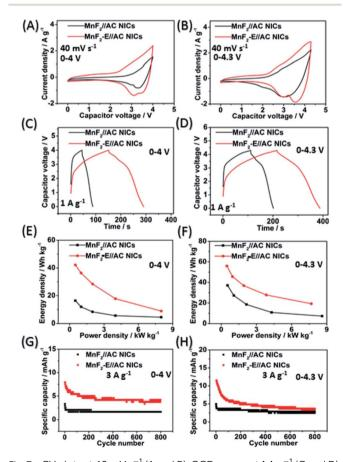
Fig. 7 CV plots at 40 mV s<sup>-1</sup> (A and B), GCD curves at 1 A  $g^{-1}$  (C and D), Ragone plots (E and F), and cycling behavior for 800 cycles at 5 A  $g^{-1}$ (G and H) of MnF<sub>2</sub> 8#//AC and MnF<sub>2</sub> 8#-E//AC NICs under the voltages of 0-4 V and 0-4.3 V, respectively.
