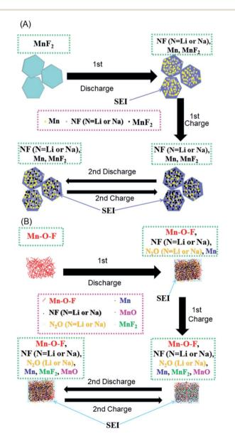
Scheme 1 Schematics of the possible reaction mechanisms for the MnF<sub>2</sub> (A) and MnF<sub>2</sub>-E (B) electrodes during the first two cycles of discharging/charging processes.
