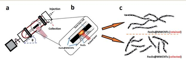
Fig. 1 Schematic illustration of the experimental procedure for the preparation for  $Fe_3O_4$ @MWCNT. (a) The vortex fluidic device (VFD) and laser Nd:YAG processing at 1064 nm. (b) Zoomed in schematic for generating  $Fe_3O_4$  NPs under laser irradiation of an iron rod (power at 250 mJ). (c)  $Fe_3O_4$ @MWCNT exiting the tube under continuous flow (collected) and retained in the tube.
