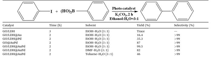
Reaction conditions: iodobenzene, 1 mmol; phenylboronic acid, 1.5 mmol; photocatalyst, 0.01 g; base: K<sub>2</sub>CO<sub>3</sub>, 3 mmol; 20 mL of solvent (V:V = 3:1);  $25 \pm 5$  °C for 2 h.
