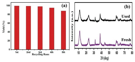
Fig. 8 (a) A reusability study over five successive runs of the SCR using the GO/LDH@AuPd nanocomposite, and (b) XRD patterns of GO/ I DH@AuPd before and after the photocatalytic reaction
