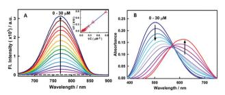
Fig. 1 (A) Fluorescence spectra of 15  $\mu$ M stryl-11 with increasing concentration of insulin fibrils (0–30  $\mu\text{M})$  [ $\lambda_{ex}$  = 630 nm]. Inset shows the double reciprocal plot (1/F vs. 1/C) and the solid line represents the fitting of the data points according to the 1:1 binding model. (B) Absorption spectra of 15  $\mu M$ stryl-11 with the increase in concentration of insulin fibrils (0-30  $\mu$ M)
