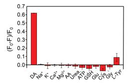
Fig. 4 Relative fluorescence decrement ( $(F_0 - F)/F_0$ ) of the bioprobe (15  $\mu$ g mL<sup>-1</sup>) in the presence of different interfering substances.  $F_0$ : Fluorescence intensity of the blank, F: fluorescence intensity of the bioprobe upon the addition of the inspected species. Dopamine: 10  $\mu$ M, Na<sup>+</sup>/K<sup>+</sup>: 1 mM, L-Tyr: 10  $\mu$ M, other substances: 100  $\mu$ M.
