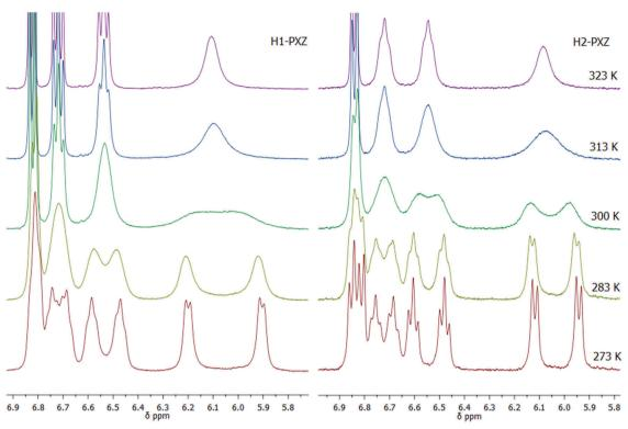
Fig. 1 Variable temperature <sup>1</sup>H NMR experiments for H1- and H2-PXZ at 273-323 K in chloroform-d, showing the aromatic peaks in the range 5.8 to 6.9 ppm.
