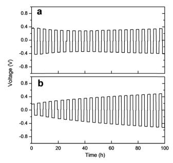
Fig. 6 Galvanostatic cycling of (a) the Li/LZP/Li symmetric cell, (b) the Li/LZP/Li symmetric cell using Au buffer, at 80  $^{\circ}\text{C}$  and 40  $\mu\text{A}$  cm $^{-2}$  current density.
