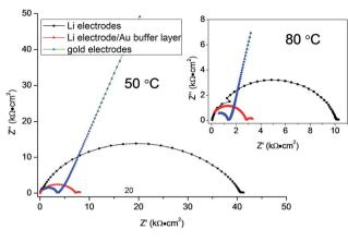
Fig. 4 Impedance plots of LZP-1100 using different electrodes at 50  $^{\circ}\text{C}$  (pellet thickness = 1.5 mm). The inset shows the spectra collected at 80  $^{\circ}\text{C}.$
