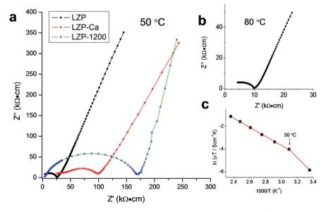
Fig. 3 (a) Typical impedance plots of LZP-1100, LZP-Ca and LZP-1200 at 50  $^{\circ}$ C using Au electrodes. (b) Impedance plot for LZP-1100 at 80  $^{\circ}$ C using Au electrodes. (c) Arrhenius plot for the total conductivity of LZP-1100 in the temperature range 25–150  $^{\circ}$ C.
