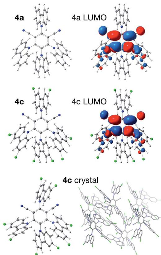
Fig. 2 Optimized structures and LUMO plots (isovalue 0.02) of the dyes **4a** and **4c** at the PBE0/def2-SVP level, as well as the crystal structure of **4c**. See the SI for the plots of **4b** and **4d**.
