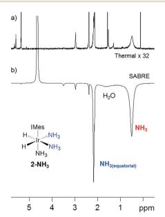
Fig. 1 (a) The thermally polarised  $^{1}$ H NMR SABRE spectrum (× 32 vertical expansion) recorded of 2-NH<sub>3</sub> (formed by reaction of 1 with NH<sub>3</sub> and H<sub>2</sub>) in dichloromethane- $d_2$  at 298 K. (b) The corresponding SABRE polarised 9.4 T  $^{1}$ H NMR spectrum after transfer under p-H<sub>2</sub> at 60 G. The hyperpolarised responses of free NH<sub>3</sub> and Ir-NH<sub>3(equatorial)</sub> of 2-NH<sub>3</sub> and residual H<sub>2</sub>O are indicated.
