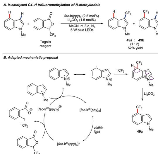
Scheme 23 Trifluoromethylation of indoles under photoredox conditions.
