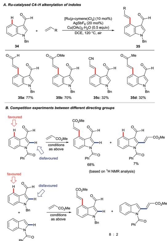
Scheme 7 Ru(II)-catalysed C4 alkenylation of 3-formyl indoles.
