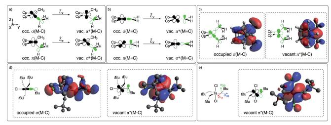
Fig. 4 (a) Main orbital contributions to the paramagnetic term for  $\delta_{11}$  in  $Cp_2M(CH_3)_2$  and (b) in  $Cp_2Ti(CH_2)$ . Frontier molecular orbitals leading to deshielding in (c)  $Cp_2M(CH_3)_2$  (M = Ti or Ta<sup>+</sup>) and (d)  $TaCl(CH_2tBu)_4$  (see Fig. 2 for orientation of CST). (e) CST orientation and LUMO of  $TaCl_2(CH_2tBu)_3$ .
