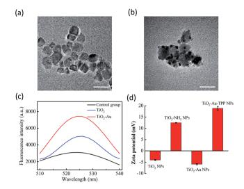
Fig. 1 Characterization of the nanoradiosensitizers. HRTEM images of the (a)  $TiO_2$  NPs and (b)  $TiO_2$ –Au NPs; the scale bars are 20 nm. (c) Fluorescence spectra of DBZTC (excitation = 490 nm, emission = 525 nm) after irradiation with X-rays. (d) Zeta potentials of each step of the modification:  $TiO_2$  NPs;  $TiO_2$ –NH<sub>2</sub> NPs;  $TiO_2$ –Au NPs; and  $TiO_2$ –Au–TPP NPs.
