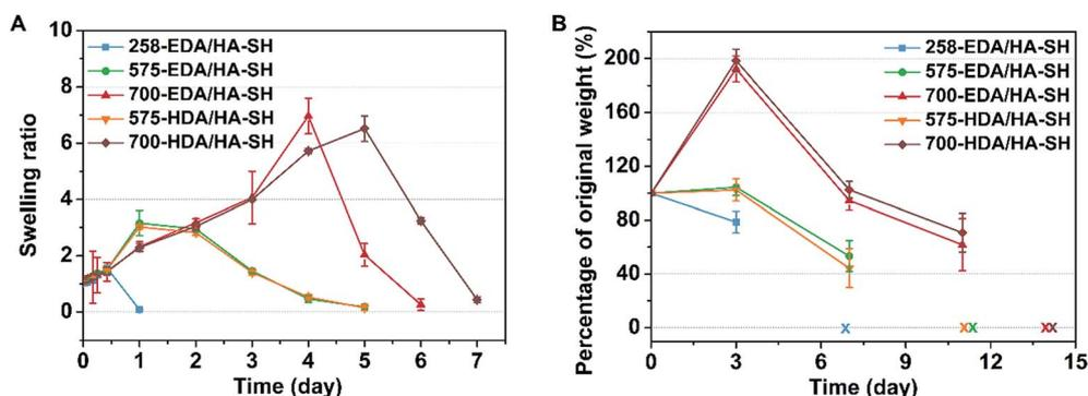
Fig. 3 The degradation profile of HP-PBAE/HA-SH hydrogels. (A) The swelling ratio of the hydrogels in PBS at 37 °C ( $n = 4$ ). (B) The *in vivo* degradation by subcutaneous implantation. The "X" represents the time at which the hydrogels totally disappeared ( $n = 4$ ).
