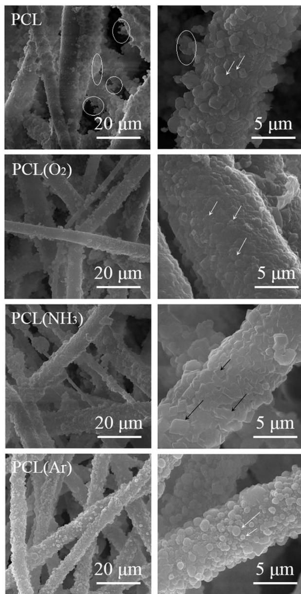
Fig. 3 SEM images of PCL/CaCO<sub>3</sub> scaffolds before and after plasma treatment at different magnifications.
