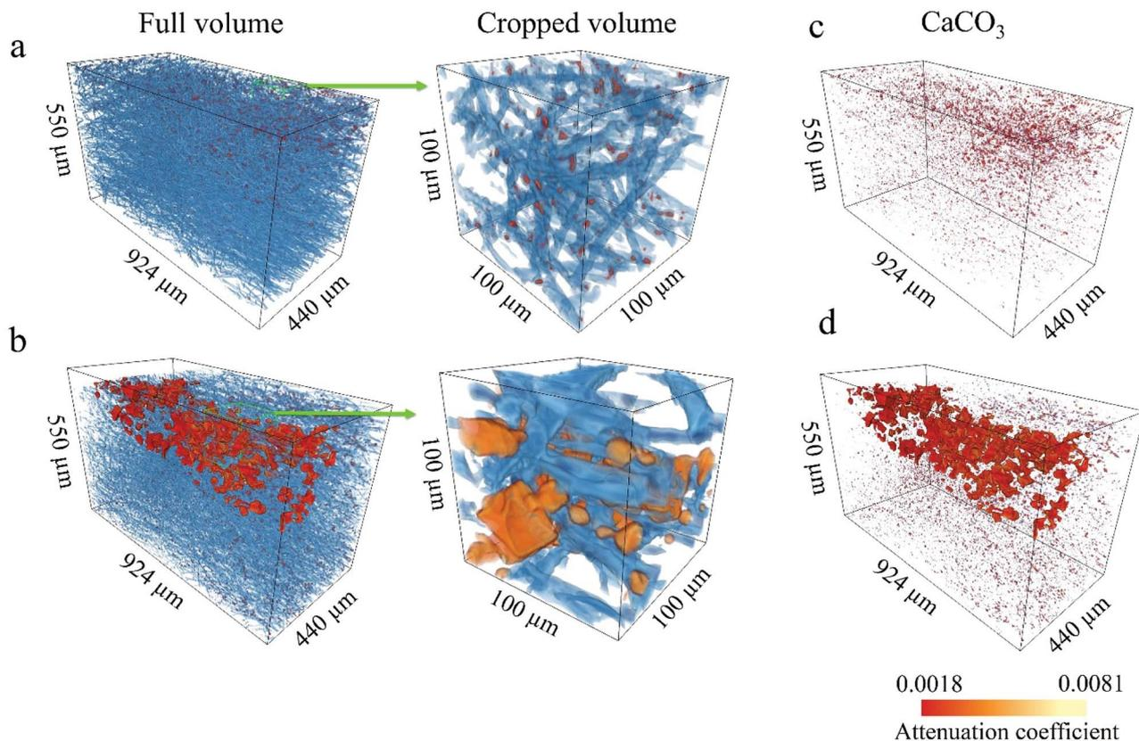
Fig. 5 X-ray- $\mu$ CT-based visualisation of full and cropped volumes of untreated PCL/CaCO<sub>3</sub> scaffolds (a and c) and PCL/CaCO<sub>3</sub> scaffolds after O<sub>2</sub>-plasma treatment (b and d) and CaCO<sub>3</sub> distribution within the volume of 3D scaffolds (c and d). The polymer and inorganic phases are shown in blue and red-yellow colours, respectively. The colour bar represents the X-ray linear attenuation coefficient in  $\mu\text{m}^{-1}$ .
