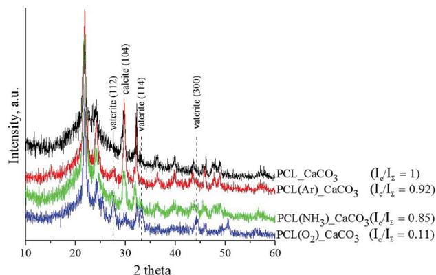
Fig. 4 XRD spectra of PCL/CaCO<sub>3</sub> scaffolds before and after plasma treatment. The ratio of the integrated intensity of the calcite phase ( $I_c$ ) to the total integrated intensity ( $I_{\Sigma}$ ) represents the relative proportion of the calcite phase in the deposited coatings.
