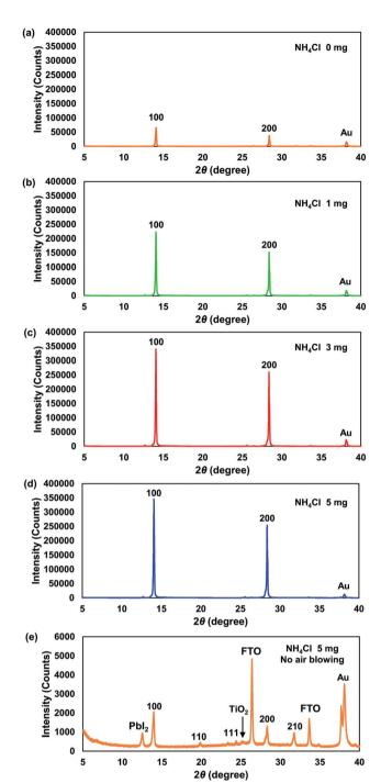
Fig. 7 XRD patterns of  $CH_3NH_3PbI_3(CI)$  cells containing (a) 0 mg, (b) 1 mg, (c) 3 mg, and (d) 5 mg of  $NH_4CI$ , and (e) XRD pattern of the  $CH_3NH_3PbI_3(CI)$  cell containing 5 mg of  $NH_4CI$  without air blowing.
