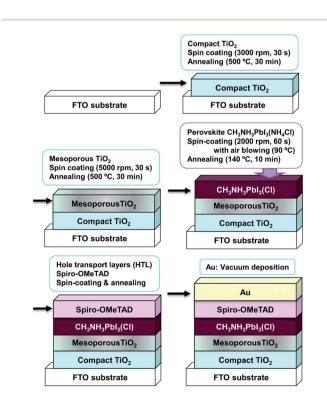
Fig. 1 Schematic illustration of the process used to fabricate the CH3NH3PbI3(CI) photovoltaic cells.
