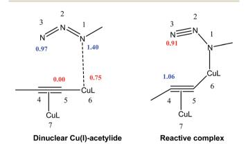
Fig. 3 Local nucleophilicites  $N_k$ , (in eV in blue) and local electrophilicites  $\omega_k$  (in eV in red) calculated using Parr function.
