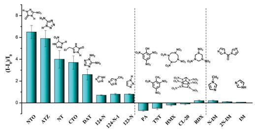
Fig. 3 Fluorescence enhancement  $((I - I_0)/I_0)$  of **E,E-HPB-ID** by different analytes  $(M_{E,E-HPB-ID}: M_{analytes} = 1:2)$  in the 90% water fraction in THF/water mixtures. [**E,E-HPB-ID**] =  $1 \times 10^{-4}$  mol L<sup>-1</sup>.
