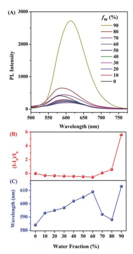
**Fig. 1** (A) Photoluminescence (PL) spectra of **E,E-HPB-ID** in THF/water mixtures. (B) Correlation between the net change in PL intensity  $[(l-l_0)/l_0]$ , and (C) the wavelength of **E,E-HPB-ID** with different water fractions in the THF/water mixtures. [**E,E-HPB-ID**] =  $1 \times 10^{-5}$  mol L<sup>-1</sup>; excitation wavelength: 410 nm.
