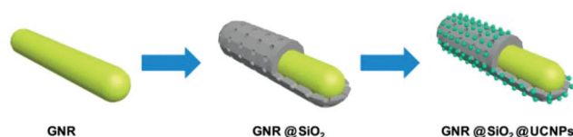
Scheme 1 Schematic illustration of the synthetic procedure for the preparation of the GNR@SiO 2 @UCNPs nanocomposite.
