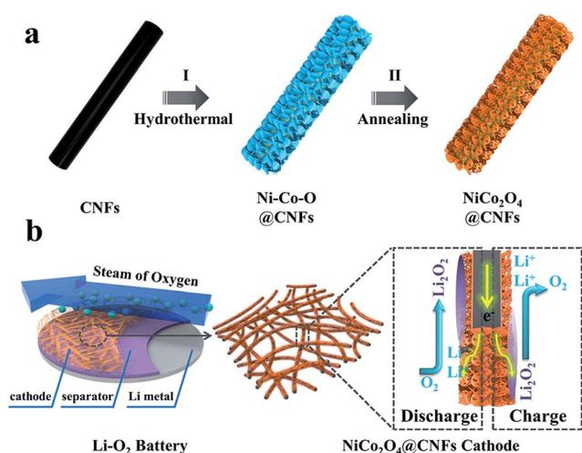
Fig. 1 (a) Schematic illustration of the fabrication of the NiCo<sub>2</sub>O<sub>4</sub>@CNFs cathode; (b) structure of the rechargeable Li–O<sub>2</sub> battery containing this cathode.
