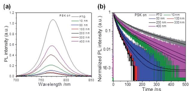
Fig. 5 (a) PL spectra and (b) PL decay profiles of PSK, and PSK deposited on varied compact ALD-TiO<sub>2</sub> HBL films. The PL spectra were obtained at excitation wavelength 633 nm; the transient PL decays were obtained using TCSPC with excitation at 635 nm and probe at 770 nm. The fitted results are represented in black lines for all results.
