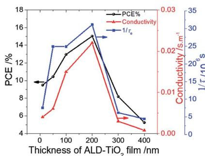
Fig. 6 Correlation of device performance (PCE/%) (black) with the thickness of an ALD-TiO<sub>2</sub> film with respect to conductivity/ $\text{S m}^{-1}$  (red) and rate of interfacial electron transfer ( $1/\tau_c/\text{s}^{-1}$ ) (blue).
