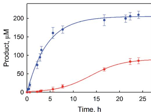
Fig. 1 Time courses of the products [PhOH (blue) and *p*-benzoquinone (red)] obtained in the photocatalytic oxidation of benzene by O<sub>2</sub> with [Ru<sup>II</sup>(Me<sub>2</sub>phen)<sub>3</sub>]<sup>2+</sup> (1.0 mM) in the presence of a catalytic amount of **1** (1.0 µM) in an O<sub>2</sub>-saturated solvent mixture of MeCN and H<sub>2</sub>O (v/v = 23 : 2) containing Sc(NO<sub>3</sub>)<sub>3</sub> (100 mM) and benzene (1.0 M) under photoirradiation (white light) at 298 K.
