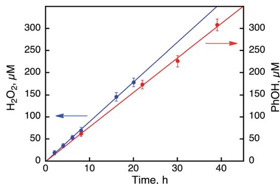
Fig. 7 Time courses of the products from the photoinduced reaction under photoirradiation (white light) in an  $\text{O}_2$ -saturated solvent mixture of MeCN and  $\text{H}_2\text{O}$  ( $v/v = 23 : 2$ ) containing **1** (0.50 mM),  $[\text{Ru}^{\text{II}}(\text{Me}_2\text{phen})_3]^{2+}$  (0.10 mM), and  $\text{Sc}(\text{NO}_3)_3$  (100 mM) in the absence (blue) and presence (red) of benzene (1.0 M) at 298 K.
