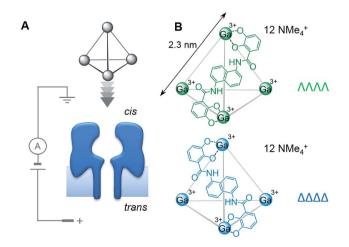
Fig. 1 (A) Experimental setup in which tetrahedral coordination cages were driven towards the  $\emph{cis}$ -opening of a single  $\alpha$ -haemolysin  $(\alpha$ -HL) nanopore inserted in a lipid bilayer under an applied transmembrane potential. (B)  $\Lambda\Lambda\Lambda\Lambda$  (green) and  $\Delta\Delta\Delta\Delta$  (blue) homochiral forms of the Ga(III) cage used in this study. Each grey edge indicates the position of a bridging ligand molecule.
