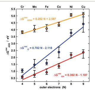
Fig. 2 Adsorption-energy trends of \*O (blue), \*OH (red) and \*OOH (orange) under vacuum for metal centers from Cr to Cu as a function of their number of outer electrons (N). The points are the average adsorption energies and the error bars show the energetic effect of the ligands in Fig. 1.
