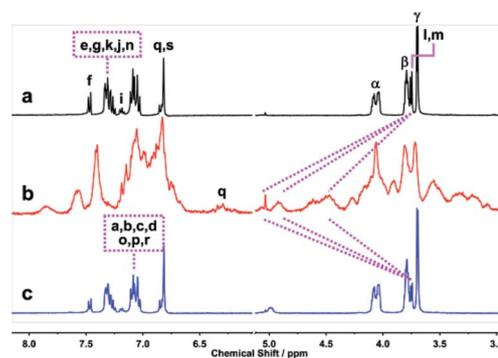
Fig. 2 Partial  $^1\text{H}$  NMR spectra (400 MHz,  $\text{CD}_2\text{Cl}_2$ , (a) of 0.5 mM 4DB24C8-TPE and 1.0 mM *E*-2DBA-TPE, (b) obtained by adding 2.4 equivalents of  $\text{HPF}_6$  to the solution of (a), and (c) obtained by adding 2.8 equivalents of  $\text{P}_1\text{-tBu}$  to the solution of (b).
