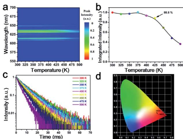
Fig. 4 (a) Temperature-dependent emission spectra of  $\text{K}_2\text{LiGaF}_6:\text{Mn}^{4+}$  from 300 K to 500 K, (b) PL integrated intensity, (c) decay time and (d) CIE chromaticity coordinates of  $\text{K}_2\text{LiGaF}_6:\text{Mn}^{4+}$  from 300 K to 500 K.
