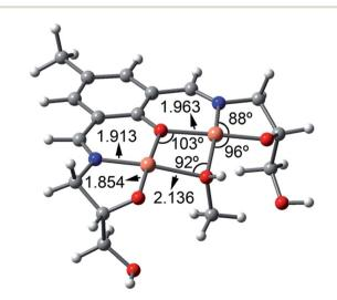
Fig. 7 BP86-D3/def2-TZVP optimized structure of  $[Cu_2(H_2dpm) MeOH]^+$  complex. Distances are in Å.
