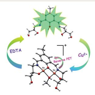
Scheme 2 Schematic illustration of proposed mechanism for the fluorescence changes of chemosensor (H5dpm) upon addition of  $Cu^{2+}$ .
