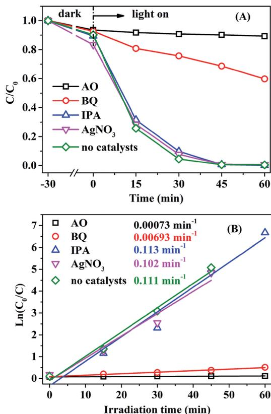
Fig. 9 Comparison of the photocatalytic performances of AMOCN3 for the degradation of RhB without adding or with the addition of ammonium oxalate (AO), benzoquinone (BQ), isopropyl alcohol (IPA), or  $AgNO_3$  under visible light irradiation.
