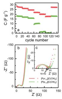
Fig. 6 (a) Specific capacitance obtained from galvanostatic chargedischarge cycling at the different rates 0.5, 1.0, 2.0, 5.0, 7.5, 10 and back to 0.5 A g<sup>-1</sup>. (b) Nyquist plots from EIS measurements and (c) inset showing high frequency semi-circle.
