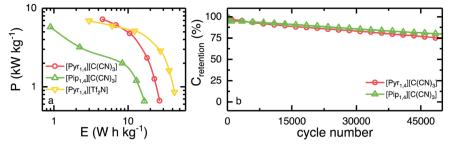
Fig. 7 (a) Ragone plot of EDLCs using  $[Pyr_{1.4}][C(CN)_3]$  (at 2.9 V, red),  $[Pip_{1.4}][C(CN)_3]$  (at 3.0 V, green) and  $[Pyr_{1.4}][Tf_2N]$  (at 3.5 V, yellow) for comparison. Values were calculated from the galvanostatic charge–discharge experiments at different specific currents, considering the electrodes active mass. (b) long-term stability of EDLCs containing  $[Pyr_{1.4}][C(CN)_3]$  and  $[Pip_{1.4}][C(CN)_3]$  operating at 2.0 A  $g^{-1}$ , from 0 V to the operating voltage.
