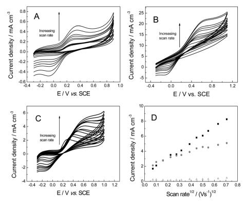
Fig. 10 Cyclic voltammetric profiles recorded for 1 mM DA in pH 7 PBS (0.1 M KCI): (A) 3D GNR, (B) 3D PTGR (C) 3D RVC electrode. (D) Depicts the analysis of voltammetric peak height vs. square-root of the applied scan rate, using 3D GNR (light grey-triangle), 3D (black-square) and 3D RVC (grey-circles) electrodes. All data obtained at a scan rate of 100 mV s<sup>-1</sup> (vs. SCE).
