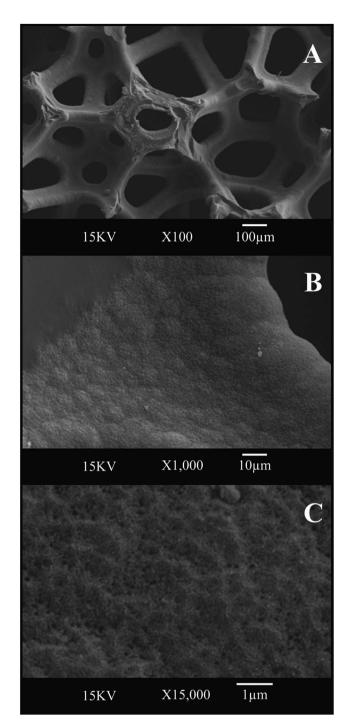
Fig. 1 SEM images of the freestanding 3D GNR foam at an increasingly higher magnification, (A)  $\times$ 100, (B)  $\times$ 1000 and (C)  $\times$ 15 000.
