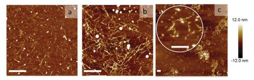
Fig. 5 Network morphology: AFM images of the sample: (a) without any cross-linker, (b) with  $r_{\rm M}=0.03$ , and (c)  $r_{\rm M}=0.095$ . The scale bars are 1000 nm.
