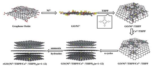
Scheme 1 Preparation procedure of rGO/(Ni<sup>2+</sup>/THPP/Co<sup>2+</sup>/THPP)<sub>n</sub>.
