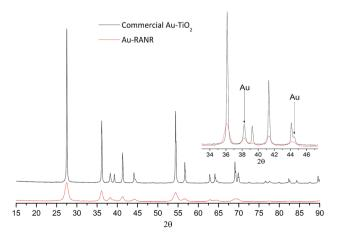
Fig. 6 PXRD patterns of 5% Au-RANR and commercial Au-TiO<sub>2</sub> after thermal treatment during catalytic cycling to 800 °C. Diffractograms of 1.2% Au loadings are shown in Fig. S12 and S13.†
