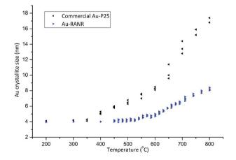
Fig. 3 Au crystallite sizes of the commercial  $Au-TiO_2$  and Au-RANR catalysts determined from Rietveld refinement from *in situ* PXRD.
