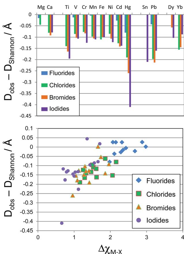
Fig. 2 Top, chart of deviation in experimental bond lengths from Shannon bond lengths in octahedral M–X bonds ( $X = \text{halide}$ ) by element. Bottom, plot of deviation in experimental bond lengths from Shannon bond lengths against difference in electronegativity.
