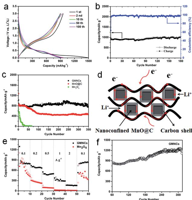
Fig. 4 (a) Discharge and charge profiles and (b) cycling performance of the GMNCs at 0.05 A g<sup>−1</sup>, (c) cycle performance of the GMNCs, MnO@C and Mn<sub>3</sub>O<sub>4</sub> at 0.1 A g<sup>−1</sup>, (d) schematic representation showing the paths for electrons and lithium-ions in the GMNCs. (e) Rate performance of the GMNCs and Mn<sub>3</sub>O<sub>4</sub> and (f) cycling performance of the GMNCs after 60 cycles rate measurement at 0.1 A g<sup>−1</sup>.
