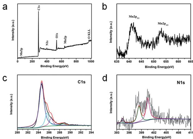
Fig. 3 XPS spectra for the GMNCs: (a) the survey spectrum and the high resolution spectra for (b) Mn2p, (c) C1s, (d) N1s.
