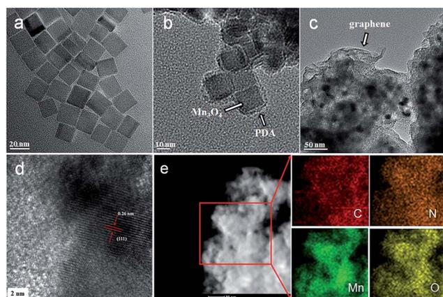
Fig. 1 TEM images of (a) the  $\text{Mn}_3\text{O}_4$  nanocrystals, (b) the  $\text{Mn}_3\text{O}_4$ @PDA nanocrystals, and (c and d) the GMNCs at different magnifications. (e) Dark-field TEM image and the corresponding EDS elemental mapping images of the GMNCs for carbon (C), nitrogen (N), manganese (Mn) and oxygen (O).
