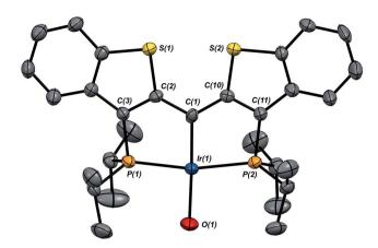
Fig. 3 Molecular structure of 3.OH. Hydrogen atoms have been omitted for clarity. Displacement ellipsoids are shown at the 50% probability level. Selected bond lengths (Å): Ir(1)-P(1), 2.2904(13); Ir(1)-P(2), 2.2817(13); Ir(1)-C(1), 1.943(5); Ir(1)-O(1), 2.004(4). Selected bond angles (°): C(1)-Ir(1)-O(1), 175.5(2); P(1)-Ir(1)-P(2), 166.08(5).
