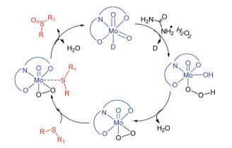
Scheme 2 Proposed mechanistic pathway for the formation of sulfoxide.
