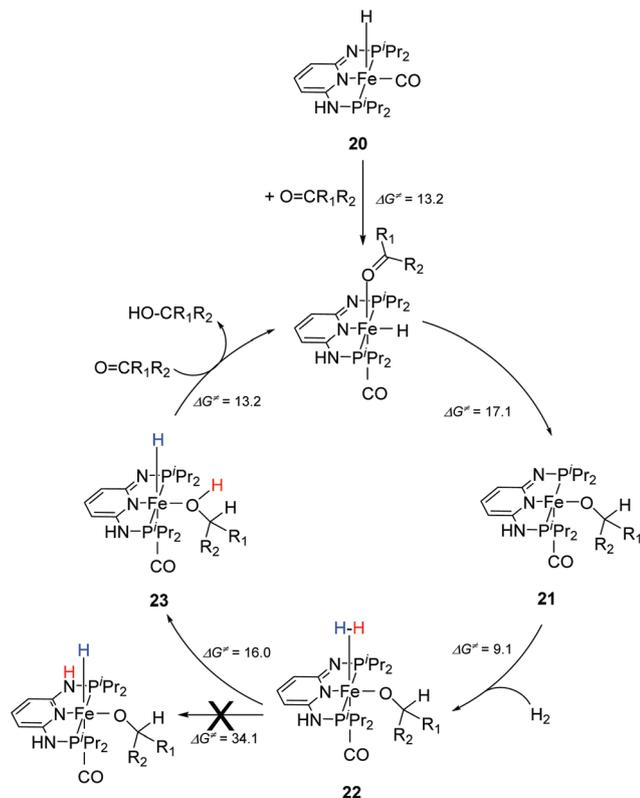
Fig. 9 Proposed catalytic cycle for the hydrogenation reactions of ketones using  $[(i^{\text{Pr}}\text{P}^{\text{N}}\text{N}^{\text{P}})\text{Fe}(\text{CO})\text{Br}]$  (**19a-Br**) as a pre-catalyst.
