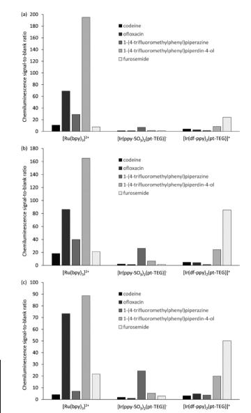
Fig. 3 Relative chemiluminescence (signal-to-blank) response for  $[Ru(bpy)_3]^{2+}$ ,  $[Ir(ppy-SO_3)_2(pt-TEG)]^-$ , and  $[Ir(df-ppy)_2(pt-TEG)]^+$  at (a) 1 mM, (b) 0.1 mM, and (c) 0.01 mM reagent concentration, with cerium(IV) sulfate (1 mM) and various pharmaceuticals and related compounds (1 μM), using flow injection analysis methodology.
