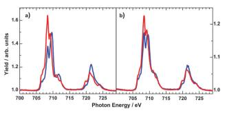
Fig. 8 Temperature-dependent iron  $L_{2,3}$  XA spectra of 4 ML of **6** on HOPG (a) and bulk powder sample crimped in indium foil (b) at 300 K (red lines) and 80 K (blue lines).
