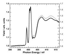
Fig. 9 N-K XA spectrum of 4 ML of  $\bf 6$  on HOPG (black line) with respect to the bulk material finely scratched onto indium foil (grey dotted line) at 300 K.
