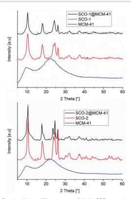
Fig. 3 Powder X-ray diffractograms of bulk SCO complexes, and SCO@MCM composite materials (background corrected). The MCM host matrix is amorphous
