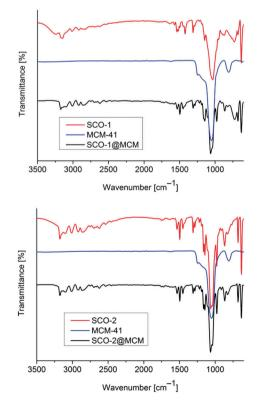
Fig. 2 IR spectra of SCO@MCM samples (black) in comparison to bulk SCO (red) and MCM-41 (blue).
